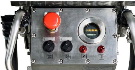
User friendly control panel with emergency stop, battery level indicator and hour counter.
