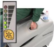
**5: Select forward traction using the illustrated switch below. Twist accelerator grip to start.**
