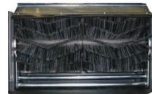
**4: Check rubber skirts around main brush for wear & damage.**
