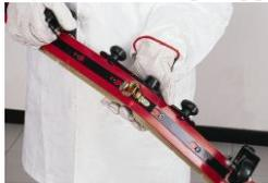
Check Rubber Edges are 'Sharp' of the blade, remember you have 4 x Edges to the blade. Squeegee Rubbers & Assembly should be Cleaned Daily, also checking for tears etc.
