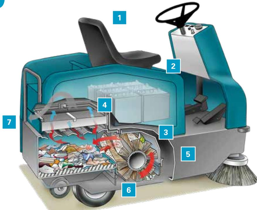
**1. Compact design** enables operators to efficiently clean in both open and congested spaces.
